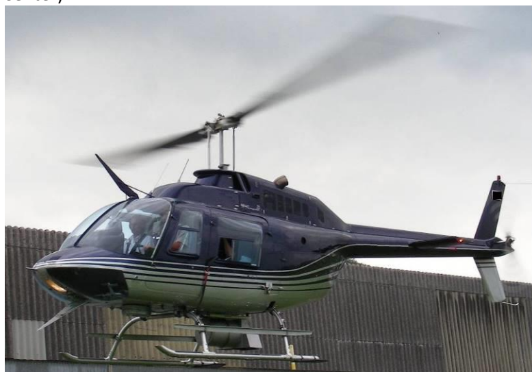
JetRanger with ALMA G2 Optical Unit (grey) Mounted to Belly
