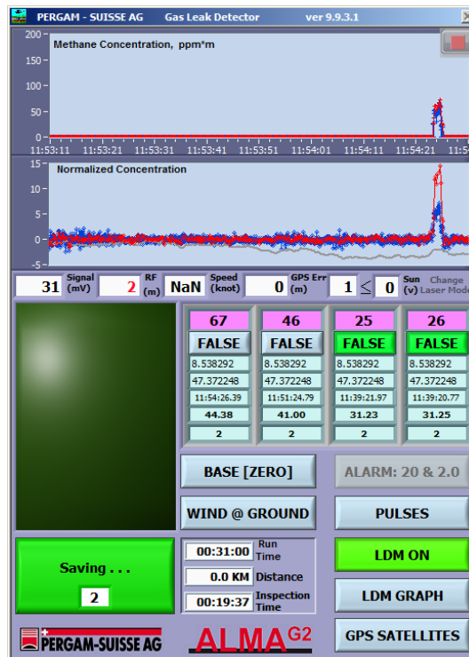
ALMA G2 On-line Software Main Screen with Leak Detection Spike
